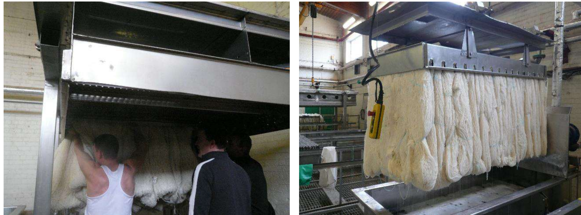
Operators need to attach the hanks from the bottom side onto the carrier for loading and remove the wet (& heavy) hanks after the dyeing process in the opposite way
