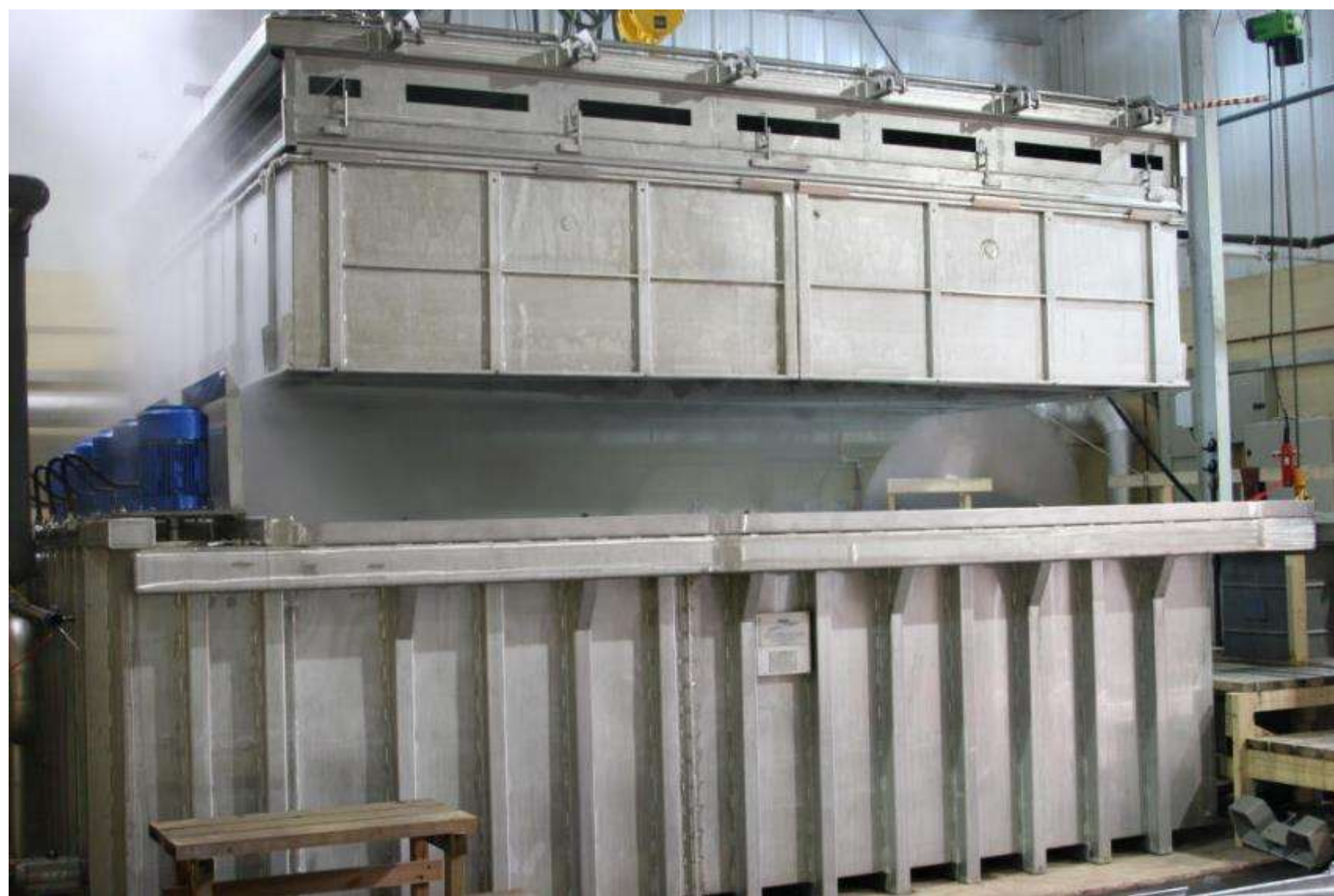
Example of 1037kg/batch dyeing system
