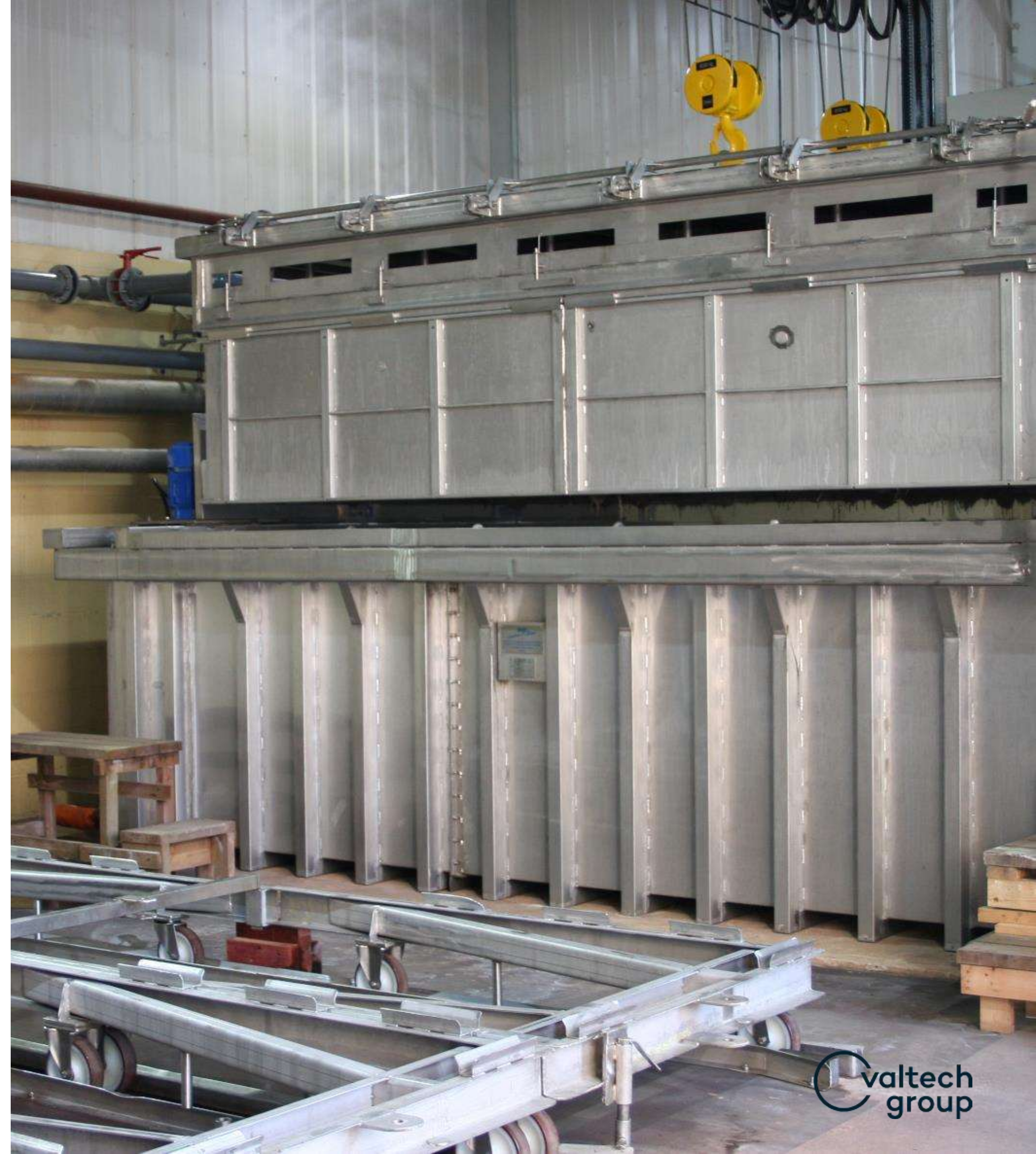
Operators need to attach the hanks from the bottom side onto the carrier for loading and remove the wet (& heavy) hanks after the dyeing process in the opposite way
