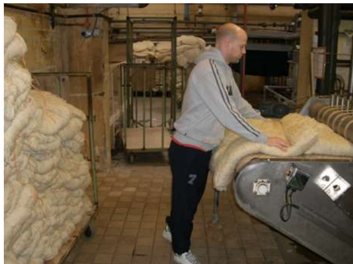
View on infeed of hank scouring line
