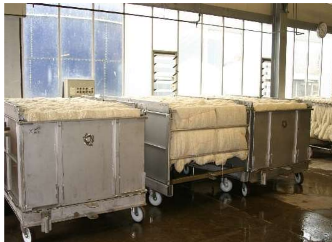
View on filled boxes at the output of the hanks scouring line
